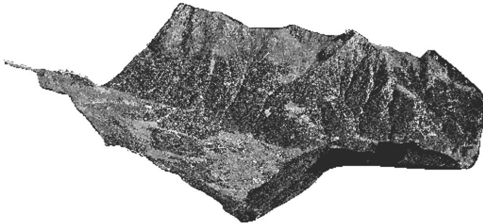
Figure 6 – 3D view of the orthophoto overlaid to the DTM of the study area.
