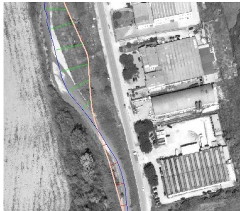
FIGURE 5.6. Bank erosion and damaging of agricultural land property: in rose the 1982 river axis path, in blue the 2001.
