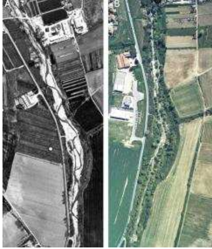
FIGURE 5.4. River bed reach showing transformation from braided to single channel morphology.
