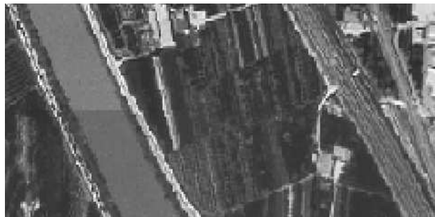
Figure 6 – Radiometric inconsistency between two adjacent orthophotos.
